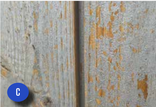
Image C shows thermally modified pine with a surface coating without EN 16755 EXT use class, resulting in the paint layer detaching from the substrate.
