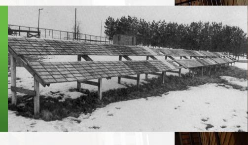
These test methods have been incorporated into standards over the world, for example, the ASTM D2898 standard in the US and EN16755 in the European Union. Available test results, both in the public domain and from manufacturers, clearly shows the same pattern in the results: It is only wood that have been treated with the polymeric flame retardant as described above that are approved for exterior use in cladding, i.e. that survives the heavy test conditions in ASTM D2898 and EN16755.
